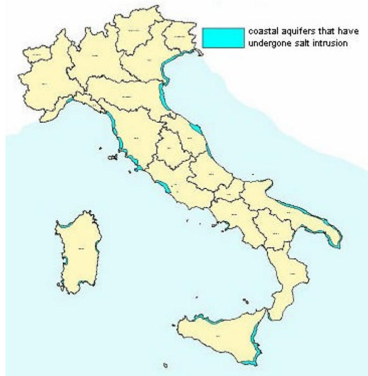
Fig. 5.1 – The main areas where coastal aquifers have undergone salt intrusion (after Civita M.V., 2005).
