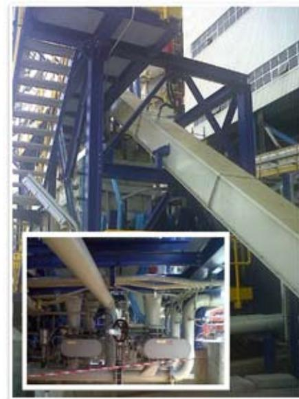
**Figura 2 - Grinding and Injection Unit.**
